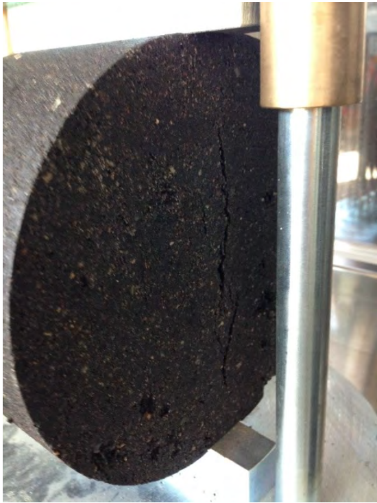
Figure A5: Cracking of Sample due to Testing of Indirect Tensile Strength.
