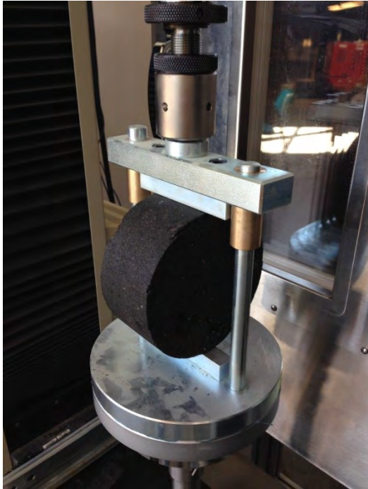
Figure A4: Compacted Sample Placed in Indirect Tensile Strength Test Apparatus.
