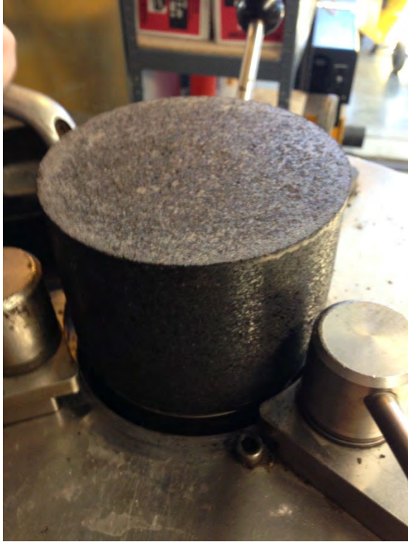
Figure A3: Slurry Trial Mix after Compaction in Gyratory Compactor.
